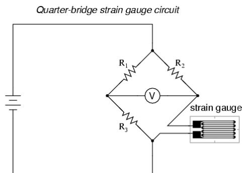
The voltage changes are extremely minute and hence we have to amplify them. We used UA741 OP-AMP to make a differential amplifier which takes the difference between the outputs and also some noise is cancelled out when the difference of the two voltages is taken. This was connected to a non inverting amplifier with a gain set to 100. The Op-Amps are powered by a constant DC supply of 9 volts each.
