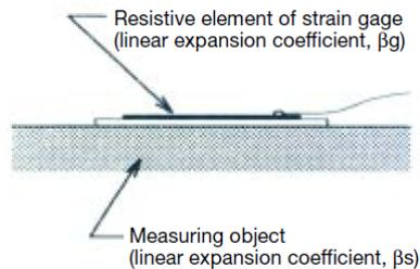
The gage factor,  $F_G$ , is determined by the material of the resistive element, and the linear expansion coefficients,  $\beta_s$  and  $\beta_g$ , are determined by the materials of
