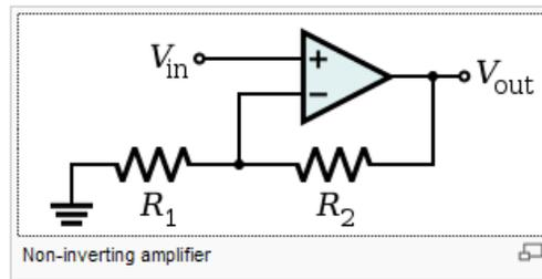
$$V_{\text{out}} = V_{\text{in}} \left( 1 + \frac{R_2}{R_1} \right)$$
